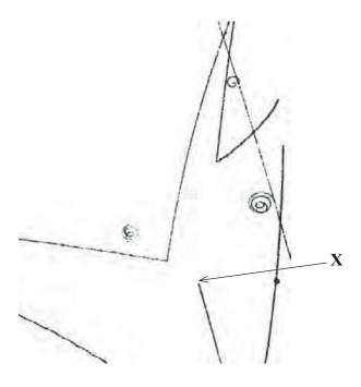
At X, an incoming charged particle interacts with a stationary proton to produce a neutral lambda particle and a neutral kaon particle. Both these particles later decay into other particles.
